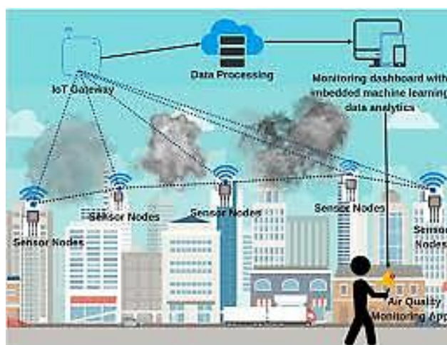
Fig. 4. Diagram of internet of things sensor nodes spread across an urban area with data routed to a central processing system.
